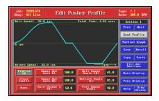
The M-2000 Integrated Pusher option allows the user to program any number of detailed sweep out motion profiles into the system to match various job requirements. The profile used for each type of ware is stored in the system job history file along with all other pusher, timing system and machine drive parameters.
