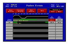
Events that relate to pusher timing can be selected and displayed on the Pusher Events screen. The timing of these events is depicted in relationship to the motion profile of the pusher sweep. This allows for accurate setup of timing for these events ahead of time rather than having to perform "trial and error" adjustments during a job change.
