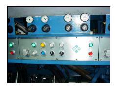
Operator controls: Two button Section Start, Gob In/Out, Blank Mold Swab, Cold Mold Cycle, Programmable Stop, Emergency Stop, Hot Ware Reject by cavity (momentary and continuous), two (2) user programmable Special Cycles and Hand Held Terminal port. The programmable Hot Ware Reject system can be controlled by the Blank Swab Cycle, Gob In/Out, Cold Mold Cycle, Special Cycles or manually.
