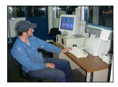
This equipment sits at the top of the M-2000 hierarchy. Twenty shops can be supervised at this level. Production information from all shops is continuously collected and stored on the system hard disk for future use. Job history files contain operational parameters for the entire complement of M-2000 equipment on each line.
