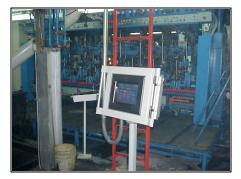
The Hot End Terminal can be optionally wall mounted or on a pedestal as shown above. All M-2000 Integrated controllers, i.e. Electronic Timing, Machine Drive and Electronic Pusher systems can be accessed via this one touch screen terminal with programmable security.
