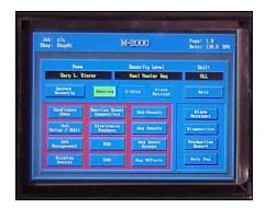
Each Integrated M-2000 controller (i.e. Electronic Timing, Machine Drive, Electronic Pushers etc.) can be monitored and controlled via this one unit. Reliable touch screen technology eliminates the need for a keyboard and pointing device on the factory floor, thus making possible greater operator efficiency.
